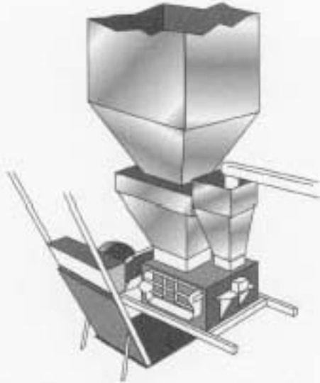
The weigh batcher is used to measure the proper amounts of each material.
